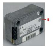
5. If needed, use the two M4 threads at the front end of the lock bolt to attach an extension.
