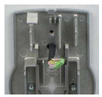
Mount battery compartment in place. Then, carefully lead the battery cable through strain relief guides of the battery compartment and the base plate.
