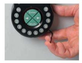
Check battery compartment for proper movability: carefully push the battery compartment into place, then slide it out again.
